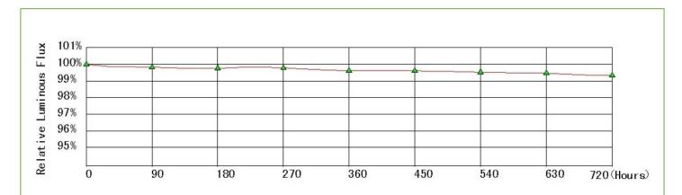
Through 720h accelerated aging test, high and low temperature prediction in the rated under the working condition after 3500h, will provide an average 70% optic maintenance ratio(L70).
